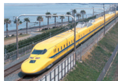
“Dr. Yellow” checks the condition of the track and overhead power supply wires.
