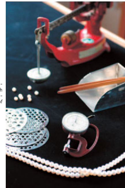
Gauges to measure the diameter and screening plates with holes named "Furui" to separate pearls by size are some of the tools for classification.
