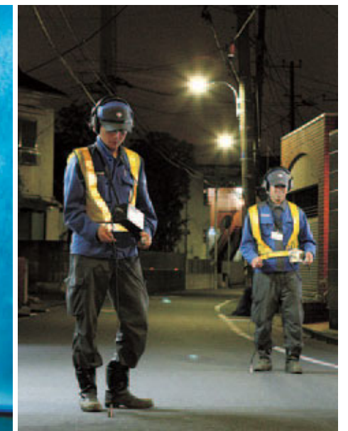
In the middle of the night, workers listen (with the help of instruments) for water leaking from underground pipes.
