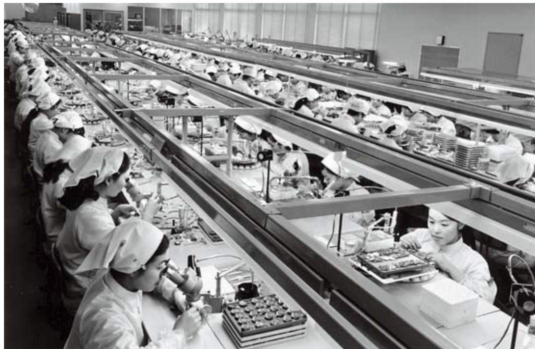
Assembly line for wristwatches at a Seiko factory around the year 1970. The number of timepieces produced in Japan grew by leaps and bounds in the 1960s and 70s, thanks to strict quality controls and efficient mass production launched by the industry in the second half of the 1950s.
