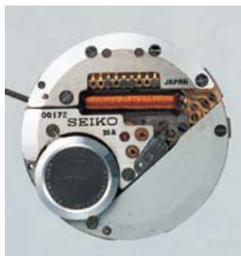
Right: The world's first quartz wristwatch was called the Quartz Astron. Made by Seiko in 1969, it surprised consumers with an accuracy within 0.2 seconds per day, or 5 seconds per month. Left: The working innards of the Quartz Astron.
