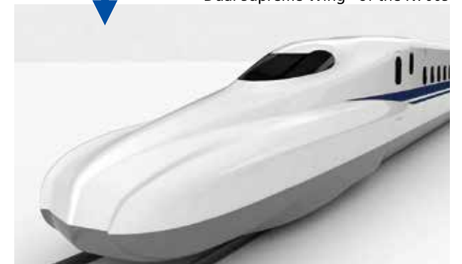
The front shape of the N700S has been evolved to cut noise and wobble for a more comfortable ride. *The position of the lights is to be determined.
