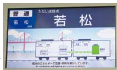
The flow of energy inside the train is displayed on an information board on the train.
