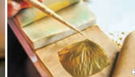
3. After transferring to another stack of foil-beating paper, this is thinned by more machine hammering.
