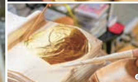
4. After being flattened to its limit, the gold leaf sheets are sorted.
