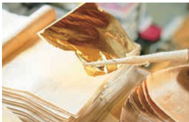
The artisan's accumulated experience and skills are indispensable to hammer gold leaf that is thin enough to be translucent.
