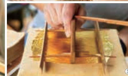
5. One sheet is trimmed at a time with a square frame-like blade.
