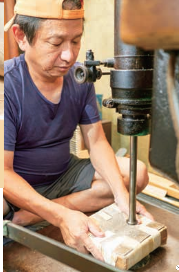
2. The bundle of paper enveloping the gold leaf is wrapped in leather and hammered with a machine.
