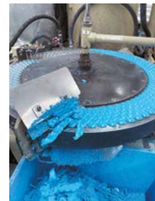
Top: Cray-Pas are made from both natural and synthetic pigments. Bottom: Cutting away the overflow of mixture from the molds at the factory. The scraps are then added back to the mixture to make more oil pastels. Photos: SAKURA COLOR PRODUCTS CORPORATION
